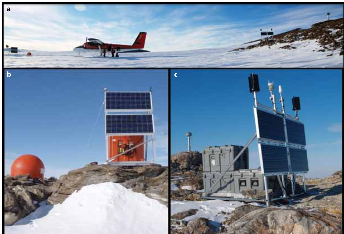
Fig. 2.8-6. POLENET autonomous, co-located continuously-recording seismic and GPS stations at Wilson Nunatak in Antarctica (a, upper panel). Seismic stations may be installed on snow, whereas GPS require bedrock, a major control on distribution of stations in polar regions. Remote sites are commonly hundreds of kilometers from logistic hubs, requiring long-range aircraft for deployment. Configurations of seismic (b, lower left panel) and GPS (c, lower right panel), show power system components (solar panels, wind turbines and extensive battery banks [in boxes]), Iridium antenna for remote communications with sensors. The GPS site has an ancillary meteorological package installed. (Photos: Antarctic POLENET field team)
